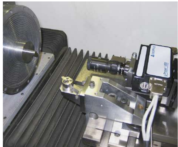
μPhase® integrated into a turning machine
