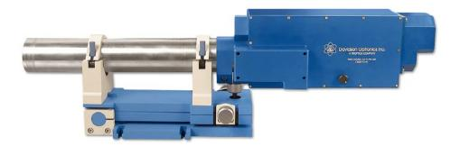
The Model D-275-AAT Automatic Autocollimating Alignment Telescope focuses from 16 inches (40cm) to infinity, to align and measure the location and angular orientation of any number of targets along its optical axis. Since the mechanical axis of the tube and the optical axis of the instrument are parallel within 3 arc seconds, the instrument is easily adaptable to mounts, jigs, stages, and various setups and setups using a dial indicator.
